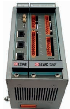
Example of small RTU7M solution – complete protection relay with wide communication abilities
